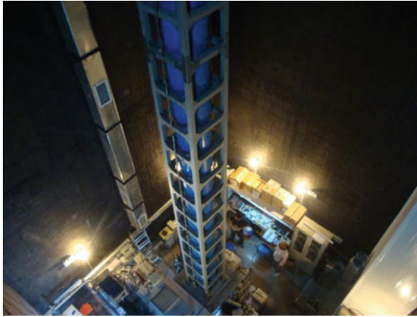
Fig. 10 The fountain tube and magnetic shielding cylinder are mounted between two MOTs
