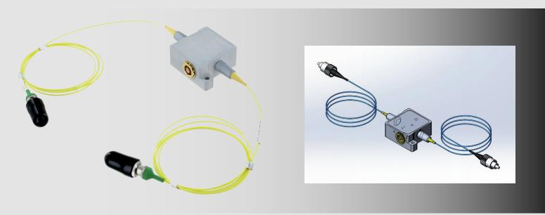
These Compact fibre pigtailed devices are **optimized for 1310 or 1550 nm.**They are made of doped glass which provide interesting features such as **insensitivity to polarization** and **low RF power consumption.** They can be used for intensity modulation as well as frequency shifting for telecommunication or remote control applications. They have been developed for industrial applications in order to offer the best performances and stability.
